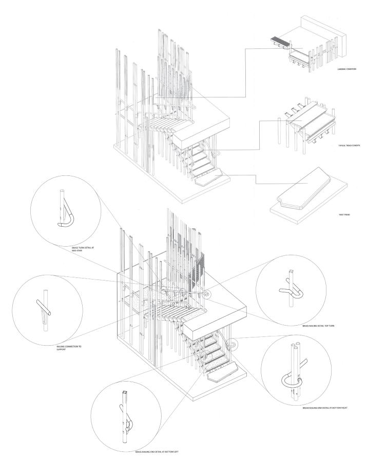
Figure 4: Digital reconstruction of Villa Mairea main stair in Revit
