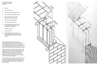
Figure 5: Replication of Ford drawing in Revit (left). Analog deconstruction of construction elements (right)..
