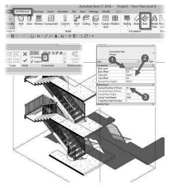
Figure 2: Revit stair tool menus and options
